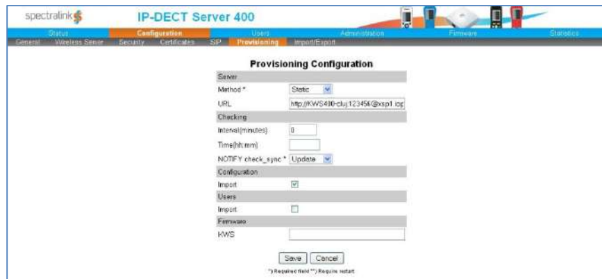
Figure 13 Example Provisioning Configuration Screen
